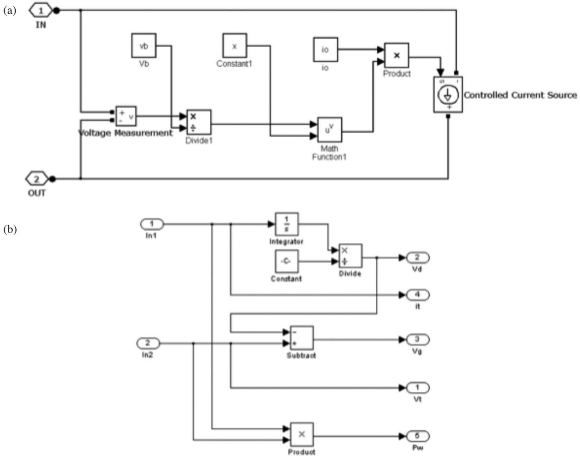
FIGURE 7. The Simulink code of (a) discharge current blocks and (b) measurement and analysis block
