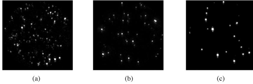
FIGURE 4. The top view of the DBD reactor operated with (a) 0.2 mm space gap, (b) 0.5 mm space gap and (c) 1.0 mm space gap
