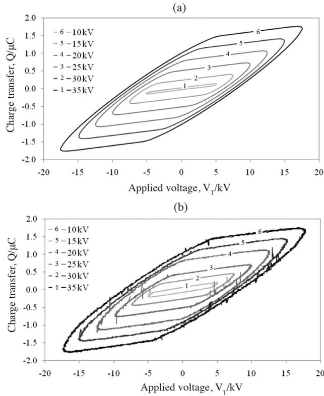
FIGURE 13. QV diagram resulting from (a) simulation and (b) experiment with 1.0 mm air gap and various applied voltages. The coefficient D and surface resistance used are 0.017 and 4.5 MΩ, respectively
