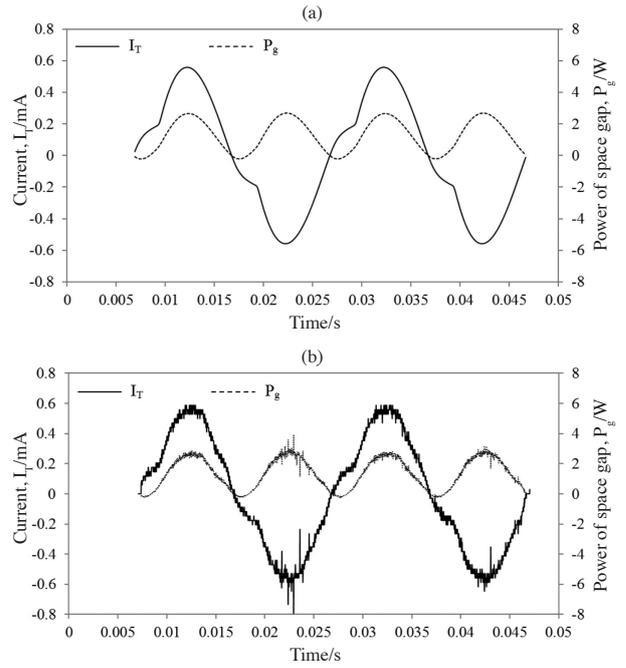
FIGURE 10. Comparison of (a) simulated and (b) experimental values of the dissipation power of space gap (dotted line) and whole discharge (black line) with 0.5 mm space gap and 30 kV pk-pk applied voltage
