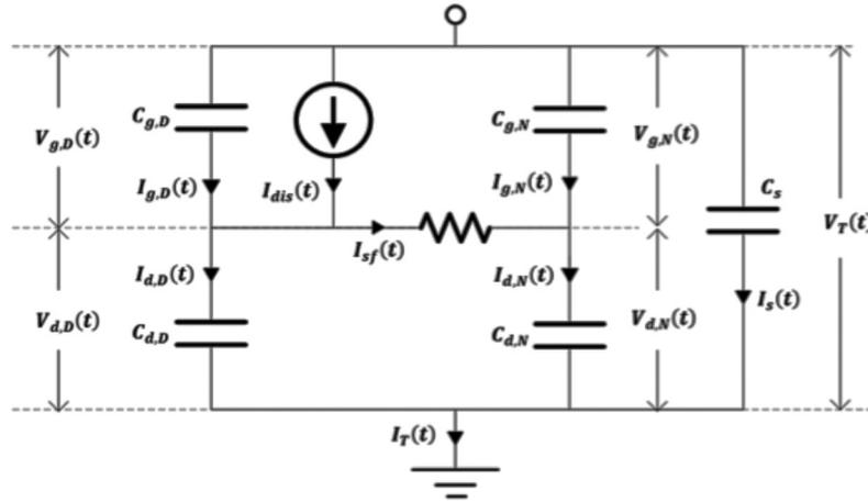
FIGURE 5. The equivalent electrical circuit of DBD indicating the discharge currents
