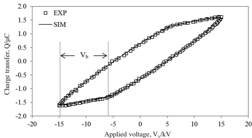
FIGURE 8. A typical QV diagram resulting from (a) simulation and (b) experiment with 0.5 mm air gap and applied voltage of 30 kV pk-pk with values of coefficient D and surface resistance 0.014 and  $2.3 \text{ M}\Omega$ , respectively
