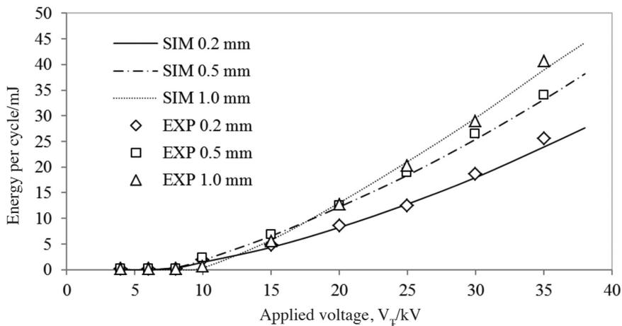
FIGURE 14. The graphs of total energy versus applied voltage with various air gaps. The lines represent the simulated results and the symbols are representing the experimental results
