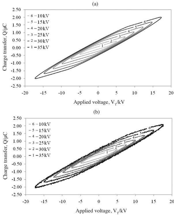
FIGURE 11. QV diagrams resulting from (a) simulation and (b) experiment with 0.2 mm air gap and various applied voltages. The coefficient  $D$  and surface resistance  $u_{sed}$  are 0.013 and 2.1  $M\Omega$ , respectively
