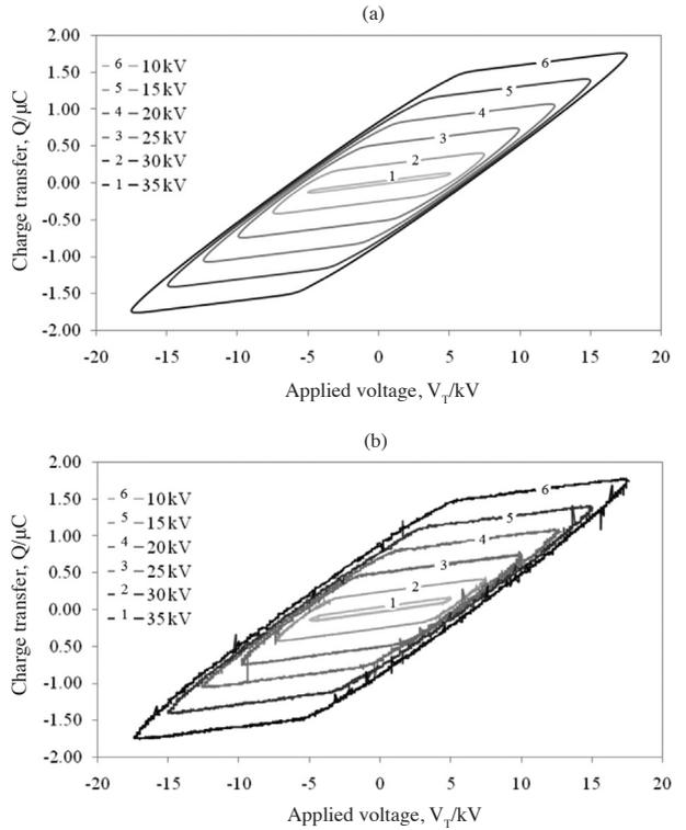
FIGURE 12. QV diagrams resulting from (a) simulation and (b) experiment with 1.0 mm air gap and various applied voltages. The coefficient  $D$  and surface resistance used are 0.017 and 1.0  $M\Omega$ , respectively
