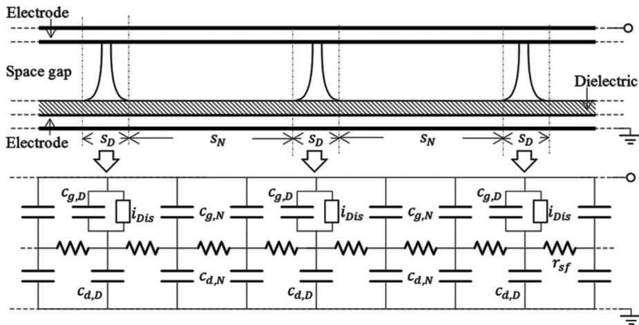
FIGURE 3. The schematic diagram showing the non-discharge region,  $S_N$  and discharge region,  $S_D$  represented in the electrical circuit
