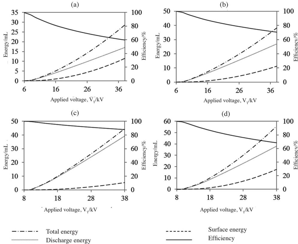
FIGURE 15. The graphs showing the simulated total energy, discharge energy, surface energy, and efficiency versus the applied voltage of smooth dielectric (a) 0.2 mm air gap, (b) 0.5 mm air gap and (c) 1.0 mm air gap. The rough dielectric with 1.0 mm air gap is shown in (d)
