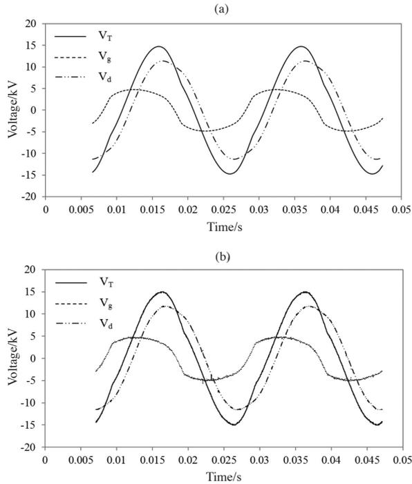
FIGURE 9. Comparison of (a) simulated and (b) experimental values of the applied voltage  $V_T$ , space gap voltage  $V_g$ , and dielectric voltage  $V_d$  for 0.5 mm air gap and 30 kV pk-pk applied voltage
