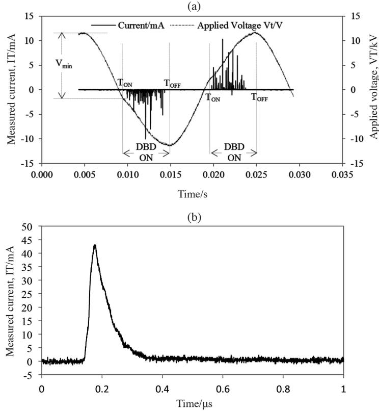
FIGURE 2. (a) A sample of DBD discharge current spikes and applied voltage.  $V_{\min}$  is pk-pk minimum breakdown voltage. The DBD is 'ON' during the time period from  $T_{\text{ON}}$  to  $T_{\text{OFF}}$ . (b) A sample of single discharge pulse in high time resolution
